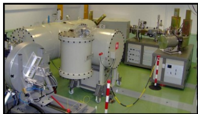
Tandem 3MV (Peleton), and 1MV (Cockcroft-Walton)
